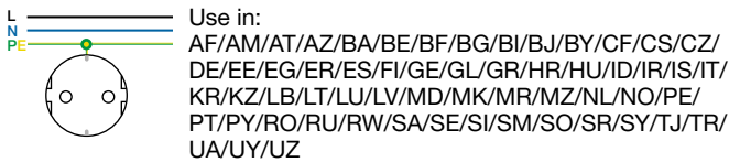
Figure 1: SCHUKO socket outlet* - 2pole + earth, 250 V~, 16 A
